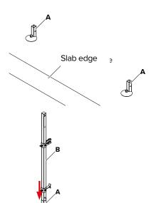
**Step 2** Insert the PROTECTO Post 130 Adjustable (B) into the PROTECTO Screw Base Joint (A).
