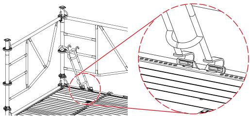
**Step 2** Raise the Deck Lifter and then attach its upper hooks to the ST 60 Frame.
