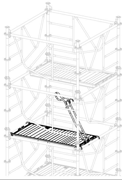
**Step 4** Hang the other end of the deck on the opposite frame. Verify that the lift-off retainer snaps into place. Remove the Deck Lifter.
