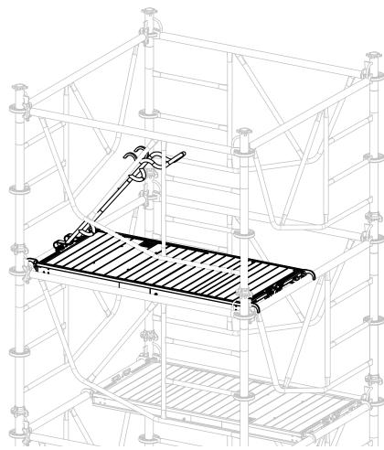
**Step 4** Hang the other end of the deck on the opposite frame. Verify that the lift-off retainer snaps into place. Remove the Deck Lifter.
