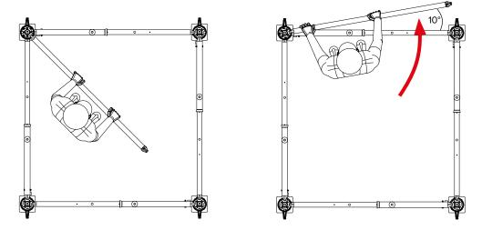
**Step 3** Place the next frame on the indicated bayonet fastener on the base frame in the same way. Pivot the frame out far enough that the rosette connection on the frame grasps the rosette on the previously attached frame.
