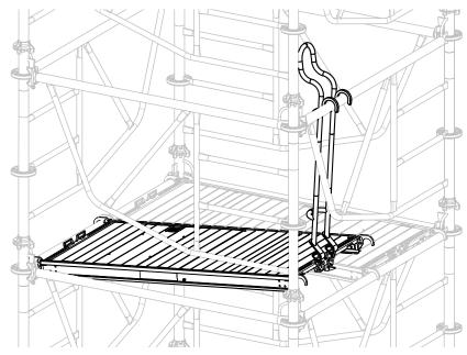
**Step 2** Use the Deck Lifter to lift the other end of the deck, then hook the Deck Lifter onto the frame of the next-higher frame level.
