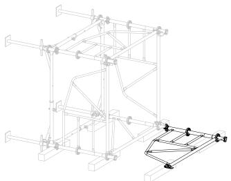
**Step 4** Place the next ST 60 Frame on the bayonet fastener shown on the ST 60 Frame of the first level at an angle of 45°.
