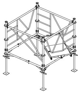
**Step 2** Slide the deck over to the opposite side, lift the deck by grasping the lift-off retainer, and hook the deck claws (**A**) onto the base frame. The lift-off retainer has to lock into place.
