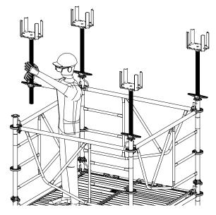
**Step 3** Place 1no. Head Jack Retainer on each Crosshead Jack to secure them from falling out, if necessary.
