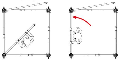
Step 4 Insert the rosette connection fixing wedge. Do not hammer in the wedge.Step 5 Attach the 2no. remaining frames in the same way, working counterclockwise.
