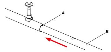
**Step 3** Press down the locking bolt. The bolt must lock completely into place and protrude from the underside of the Starter Frame L.
