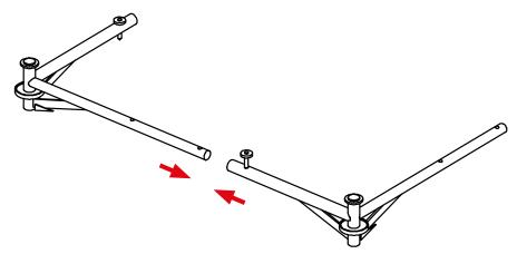
**Step 5** Put together the 2no. assembled halves of the base frame and secure them in position with the locking bolts. Two persons are required to perform this task.
