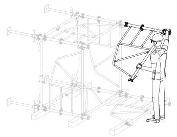
**Step 5** Pivot the frame down vertically such that the rosette connection on the frame grasps the rosette on the previously attached frame. Insert the wedge.
