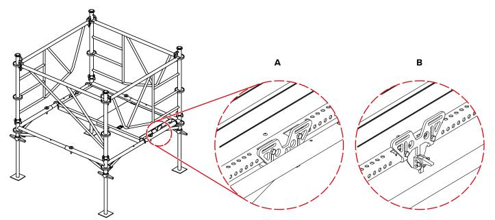
**Step 1** Insert both lower hooks of the Deck Lifter into the lift-off retainer on a deck.
