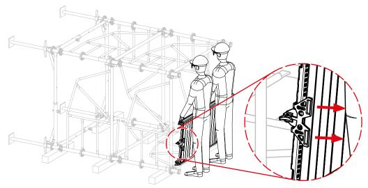
**Step 2** Press in the lift-off retainer plate and secure it, e.g. with cable ties around the outside of the ST 60 Frames (**A**).
