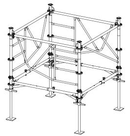
**Step 4** Turn the first unit on its side, working with two persons, and place it on boards (at least 60 mm x 60 mm). The boards should be spaced 750 mm apart (inner dimension).
