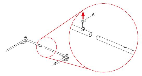
**Step 2** Put together the Starter Frames L to create the desired side lengths. The corresponding marking hole (**A** 1.50 m) or (**B** 1.13 m) should only just be completely visible.
