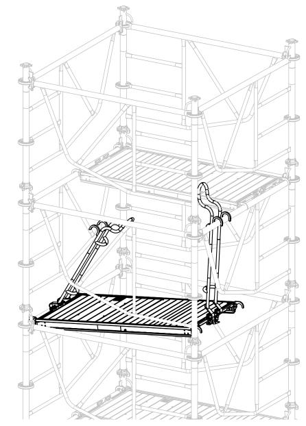
**Step 3** Hang the first end of the deck on the frame. Verify that the lift-off retainer snaps into place. Remove the Deck Lifter.
