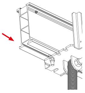
**Step 4** Slide the T Bolt into the proper groove in the Crosshead Jack.
