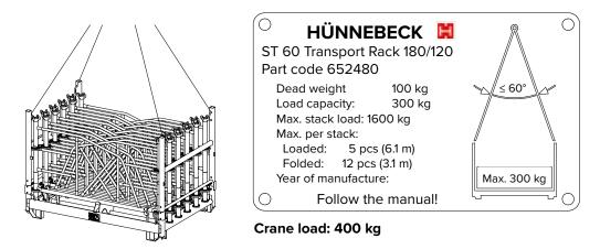
Step 2 Transport the Frame Rack 180/120 by crane.
