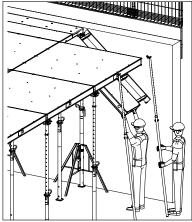
**Step 3** Place the TOPEC Adjustment Panel on the supports on the steel props.
