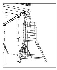
**Step 6** Working from a safe position, place the cut-to-size plywood on the telescoping piece of the TOPEC Adjustment Panel and nail to secure.
