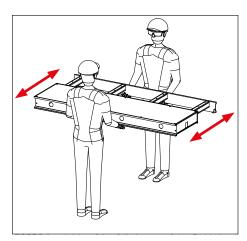
**Step 1** Assemble formwork using TOPEC Panels up to the infill area.
