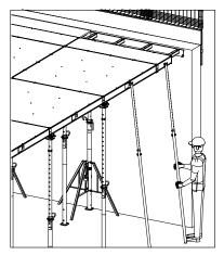
**Step 4** Use the Alu Erection Rod 365 to swivel the TOPEC Adjustment Panel to the horizontal position and rest the panel on the Alu Erection Rod 365.
