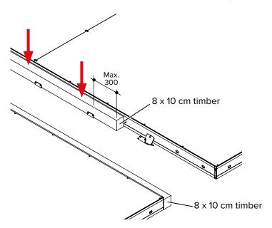
**Step 4** Secure the timber with nails.
