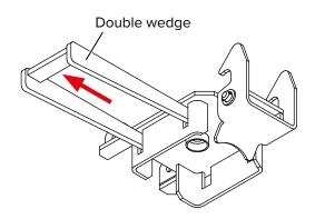
Step 7 Insert the TOPMAX GASS Multi Adapter (code:606993) with the GASS Leg attached into the folding head.
