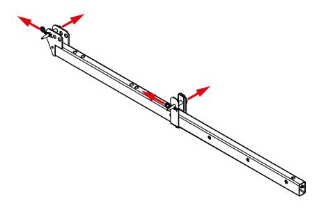
**Step 2** Position the TOPMAX Support Girder (code:603390) as per the design scheme supplied. Align the hole of the girder with the hole position of the table.
