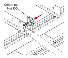
Please note the correct position of strut when attached to the "C" profiles of the TOPMAX Floor Table.
