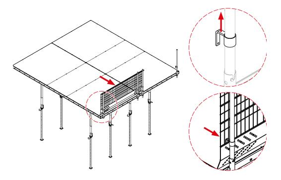
Step 6 Lower the tower board bracket and ensure that the post protrudes through the mesh at the top of the panel.
