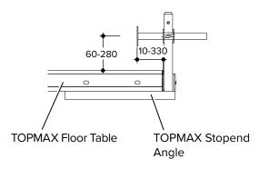
The TOPMAX Stopend Angle (code:603375) is secured to the TOPMAX Floor Table outer profile using a Centering Tension Bolt (code:479264) and a Centering Nut 100 (code:469566) located on the inside of the outer profile of the TOPMAX Floor Table (not visible below).
