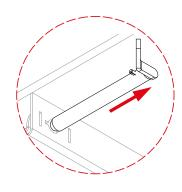
**Step 3** Slide the outriggers out to the required position.
