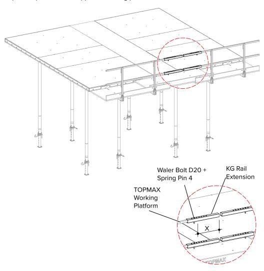
KG Rail Extensions (code:498218) are used to extend the handrails of TOPMAX Working Platform 2.4 m by X = 0.10 to 0.50 m and TOPMAX Working Platform 1.8 m by X = 0.40 to 0.50 m (measuring from the edge of the Working Platform handrail)
