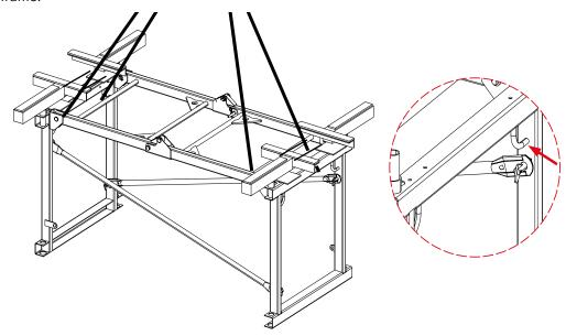
Step 9 Lift the frame into the connecting pins on top of the Multi Mover (code:607150) and secure using the Multi Mover Locking Pins (code:607156), R-safety clips not shown, at the bottom corners. The pins are ordered separately.
