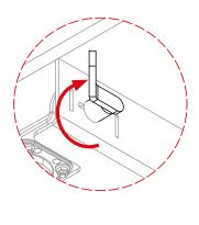
**Step 2** Pull the bolt out and keep it for later use.
