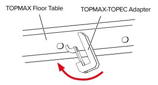
Step 2 Slot the external profile of the TOPEC panel into the exposed hook of the TOPMAX-TOPEC Adapter (code:604515) as shown in the cross-section below.
