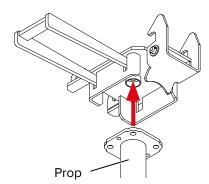
**Step 6** Push and strike the double wedge to ensure prop is securely attached.
