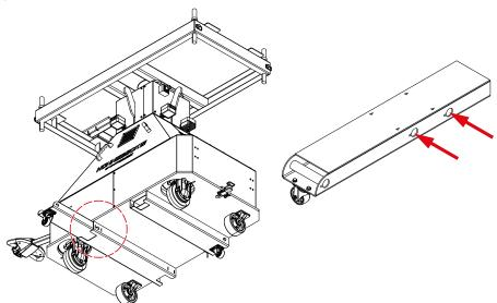
**Step 5** To secure the outrigger insert the bolt into the hole position on the rail and turn the handle bolt.
