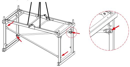
**Step 6** The crane slings can be released after the frame is securely fastened.
