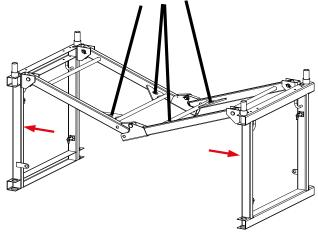
**Step 4** Fully open the extension frame and secure the hinge on each side with the locking bolts and spring pins.
