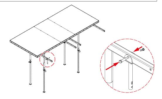
**Step 7** Insert the EUROPLUS*new* Prop in the TOPMAX Lockable Head (code:603404).
