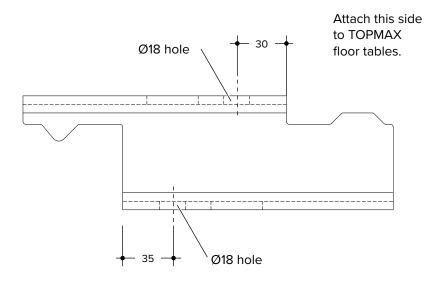
The Panel Anchor Bracket (code:605999) can be attached to TOPMAX panels as shown below to restrain the panels horizontally.
