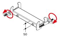
Step 2 Position the adapter on the required location along the main profile of the TOPMAX Floor Table and tighten the wing nuts again.
