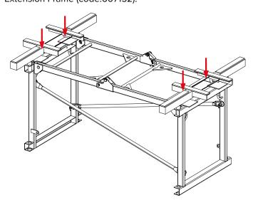
**Step 8** Attach the crane slings to the outer attachment points located on the top corners of the frame.
