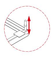
Step 3 Align the hole position on the tube with the hole position of the frame and re-insert the locking pin in the original hole position.
