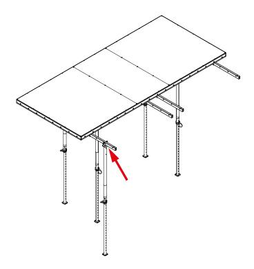
**Step 8** Secure the head using a TOPEC Bolt. For the appropriate bolt to be used see page 106.
