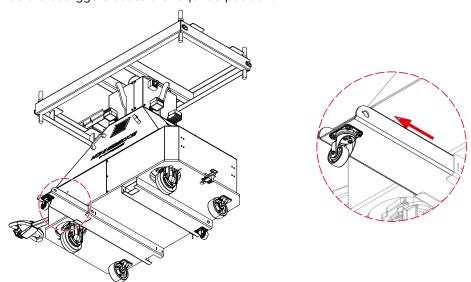
**Step 4** Align the hole positions of the outriggers with the hole of the rails, see warning on page 110.
