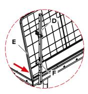
Step 7 Rotate the top of the PROTECTO Panel G2 (**E**) towards the PROTECTO Post 130 Adjustable (**D**) so that the latches capture the PROTECTO Panel G2 mesh. The PROTECTO Post latch (**G**) may require its position to be adjusted using the captive thumb screw.
