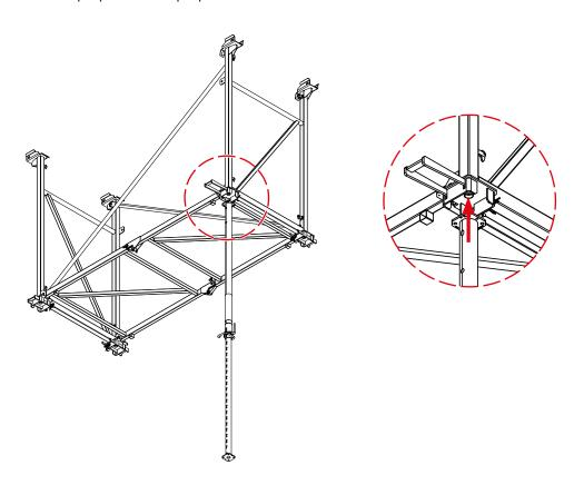
**Step 8** Secure the prop by sliding the double wedge in.
