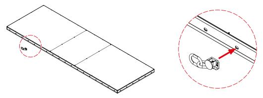
**Step 2** Insert the T bolt on the hole position. Push to ensure that the safety pin retracts.
