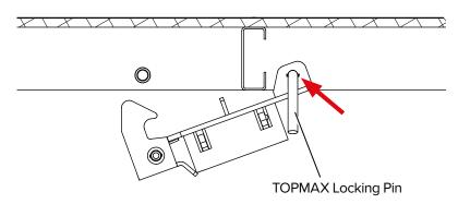
**Step 5** Swivel the head until the claw locks into the connection point on the TOPMAX Floor Table profile.
