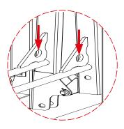
**Step 2** Once the frame is on the ground, remove both locking bolts and spring pins. Keep them for later use.
