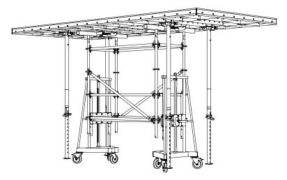
Release the props of the TOPMAX Floor Table using the quick release and slide in the inner tubes to allow the TOPMAX Positioning Unit to reach its lowest position. The integrated winches of the TOPMAX Positioning Unit allow a vertical adjustment range of 0.93 m.
