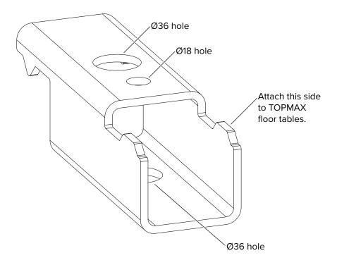
The Panel Anchor Bracket (code:605999) is secured using the Anchor Bolt MM + SSK 16 x 130 (code:443500). Only one anchor is required per bracket. To fasten the anchor bolt use a 24 mm spanner with a spanner extension.
