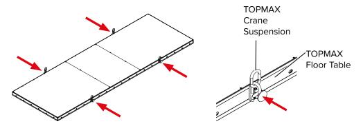
**Step 11** Attach slings to the TOPMAX Crane Suspension (code:603050) and lift the TOPMAX Floor Table.
