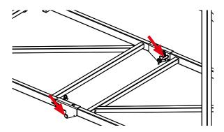
**Step 4** Brace using 2no. Diagonals 203 (code:110167) which have to be ordered separately. Secure the diagonal by hooking into the lower cross beam of the extension frame and secured to the anti-luce fittings at the top of the opposite side.
