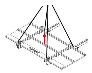
Step 3 Insert the threaded pins of the platform into the required hole positions on the external profile of the table.
