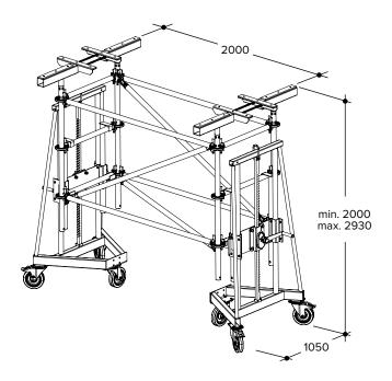
The MODEX Assembly Type 1 (loading frame) is made of the following components:
