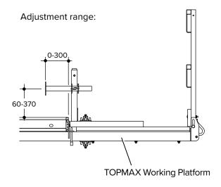
The TOPMAX Stopend Angle (code:603375) is connected to the TOPMAX Working Platform using the RASTO MP-Bolt (code:485435) through the holes of the platform and secured using 2no. Centering Nuts 100 (code:469566).
