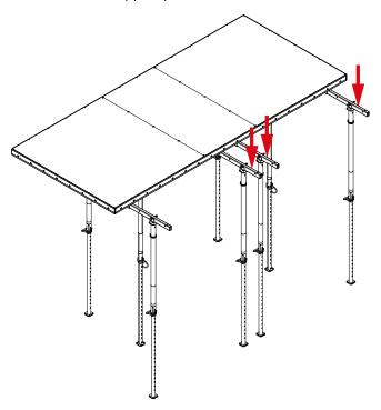
**Step 11** Position the RASTO/TAKKO Panel on top of the girders and align with the TOPMAX Floor Table.
