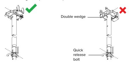
The EUROPLUS new props must be positioned so that the quick release bolts face away from the centre of the table as shown below, to prevent the quick release bolt from disengaging when swinging the props (lifting the table) and to allow the Multi Mover (code:607150) to be able to be positioned under the table.
