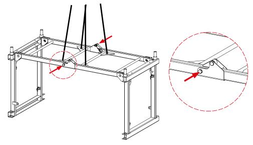
**Step 5** Attach the Guardrail 200 (code:154080) braces to the anti-luce fittings. The braces are ordered separately.
