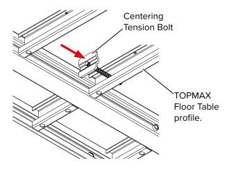
**Step 2** Insert the Wall Strut through the threaded rod of the bolt.
