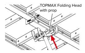
**Step 5** Swivel the TOPMAX Folding Head (code:602596) until the claw locks into the connection point on the TOPMAX Head Adapter (code:603442).
