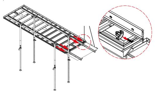
**Step 5** Once the platform is secure, release the crane slings.
