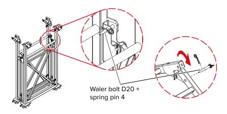
**Step 2** Unfold the frame.
