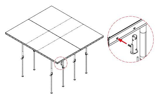
Step 2 Secure the socket base using a Centering Nut 100 (code:469566) on the inside of the external profile of the TOPMAX Floor Table.
