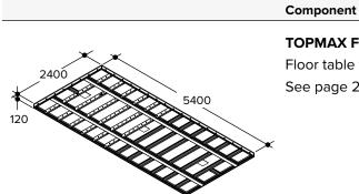
**TOPMAX Floor Table 2.4 x 5.4 m**Floor table with a forming area of 12.96 m<sup>2</sup>.
