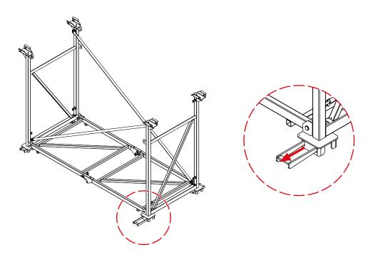
**Step 7** Attach the props onto the prop retainer of the frame.
