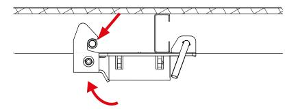
**Step 6** Pull out the double wedge of the folding head. For clarity, in steps 6–8, the table is not show.
