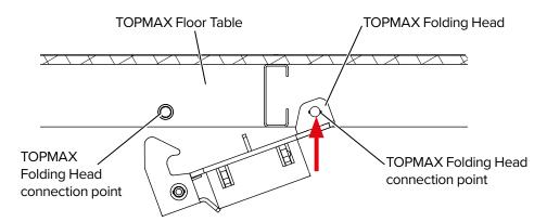
**Step 2** Insert the TOPMAX Locking Pin (code:603067) through the profile to secure the head.
