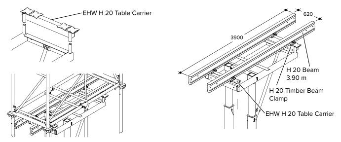
With this assembly it is also possible to pass the props with the table jack lift to pick up the table.
