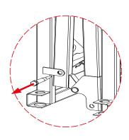
**Step 3** Whilst the Multi Mover Extension Frame (code:607152) is pulled upwards by the crane, pull the frame open by hand.
