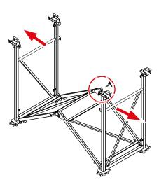
**Step 3** Insert the waler bolt D20 and secure with the spring pin 4.
