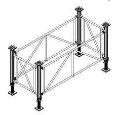
Step 2 Attach the TOPMAX GASS Tower Adapter (code:606994) to each GASS Legs using 4no. Ring Bolt Clamp for GASS Leg to GASS Leg (code:718901) per leg.
