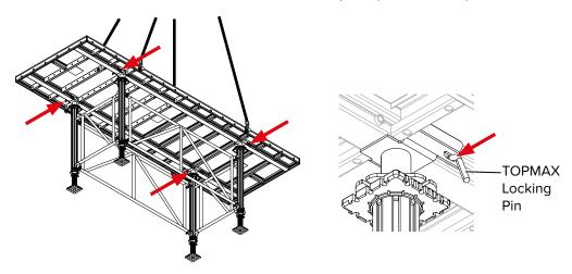
**Step 7** After checking that the table is stable, remove the crane slings and the TOPMAX Crane Suspension (code:603050).
