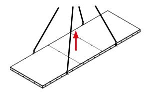
**Step 5** Position the TOPMAX Floor Table on top of the GASS frame and lower until the table is supported by the TOPMAX GASS Tower Adapters (code:606994). Align the holes in the TOPMAX main profile with the slot holes of the TOPMAX GASS Tower Adapters.
