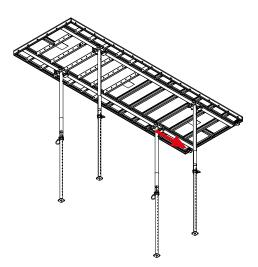
**Step 4** Insert the PROTECTO Post 130 Adjustable (**D**) into the TOPMAX Post Fastener (**A**).
