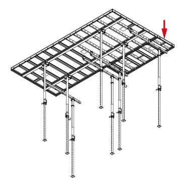
**Step 12** Insert the threaded pin of a Centering Tension Bolt (code:479264) into the required hole position on the external profile of the table.
