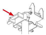
**Step 7** Swivel the head until the claw locks into the connection point on the TOPMAX Floor Table profile.
