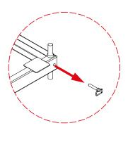
**Step 2** Adjust the height of the positioning tube.
