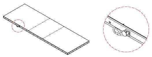
**Step 3** Rotate the TOPMAX Crane Assembly (code:603050) until the safety pin springs into the hole. A "click" sound will be audible and it will signal that the pin has been pushed out.
