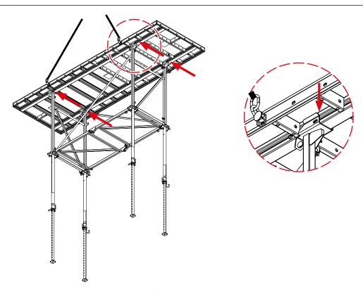
**Step 13** Secure the table by inserting the TOPMAX Locking Pin (code:603067).
