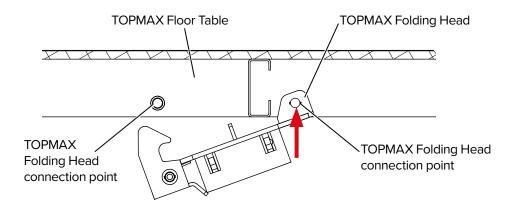
**Step 4** Insert the TOPMAX Locking Pin (code:603067) through the profile to secure the head.
