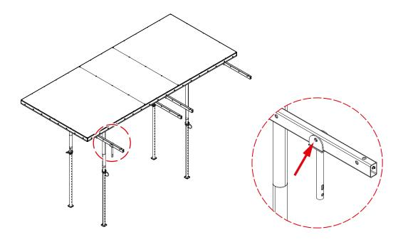
Step 6 Secure the head using a Waler Bolt D20 (code:420000) and a Spring Pin 4 (code:173776).
