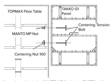
As an alternative to the MANTO MP Nut (code:454670), a Hexagon Nut 15/50 (code:164535) in combination with a Plate 8/8 (code:400214) can be used.
