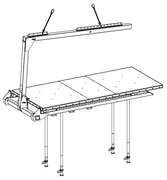
The TOPMAX Floor Table can be lifted from the short side as well as from the long side.
