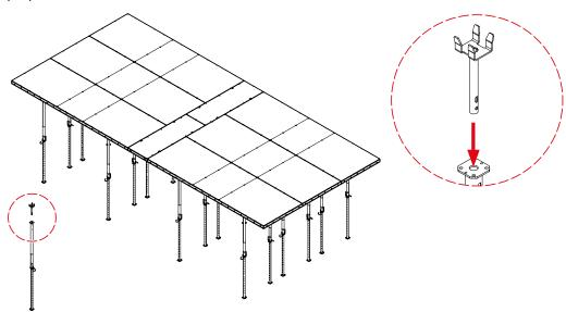
**Step 3** Secure the head using a TOPEC Bolt. For the appropriate bolt to be used see page 106.
