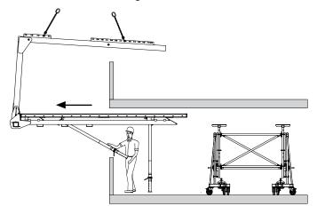
**Step 6** Release the props. The props swing back and automatically lock into place.
