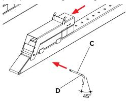
Step 3 Turn the Locking Pin grip down. The Spacer Plug Adapter is now secured to the Spacer Plug.
