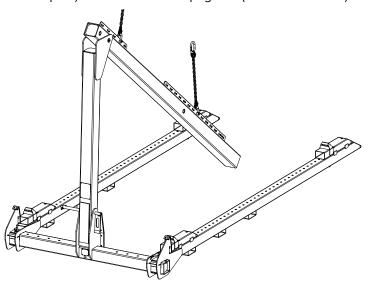
**Step 2** Attach the first fork arm to the crane at the fork arm's centre of gravity. Place a textile sling around the fork arm in a choke hitch.
