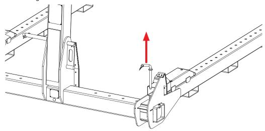
Step 5 Slide the fork arm to the desired position and secure it with the Locking Bolt. Secure the Locking Bolt with the Spring Cotter Pin.
