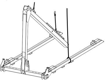
**Step 3** Raise the fork arm enough that it can easily be moved along the Cross Beam.
