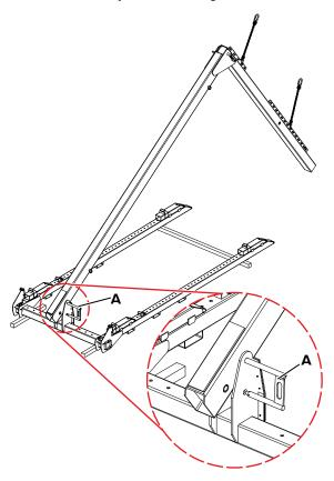
**Step 3** Attach one end of the crane lifting gear to the last hole in the long suspension rail on the Traverse Beam (**B**).
