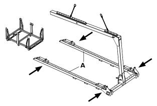
Step 2 Lift the Lifting Fork and place it in the Stacking Frame. Verify that the front forklift lugs (B) rest against the base frame of the Stacking Frame.
