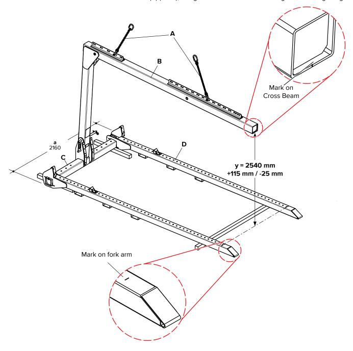
Check dimension of chain sling (A) pursuant to DIN EN 818-6:
