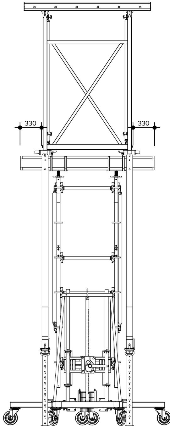
**Step 3** Load the Table Form onto the Positioning Unit and move it as described in section 8.2 on page 45. Grasp only the steering rods to move the Lifting Jack Carriages!
