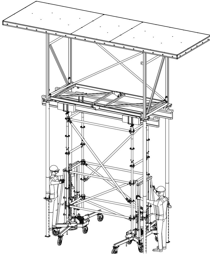
**Step 4** Load the Table Form onto the Positioning Unit and move it as described in section 8.2 on page 45. Grasp only the steering rods to move the Lifting Jack Carriages!
