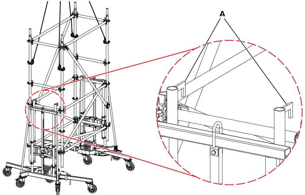
**Step 2** Push the vertical tracks down until the hooks rest on the tube ledgers (B) on the MODEX Assembly.
