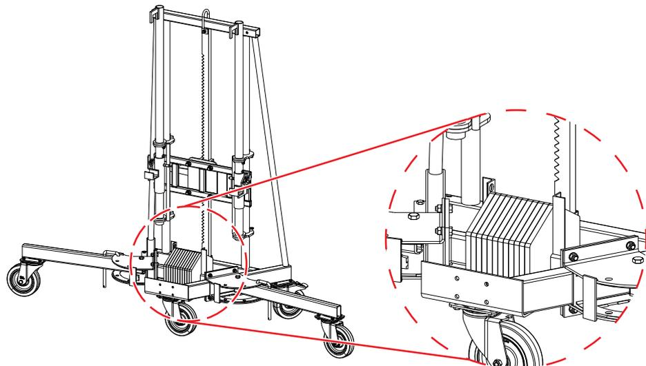
**Step 4** Slide the securing rod through the L-profiles and secure with the spring pin.
