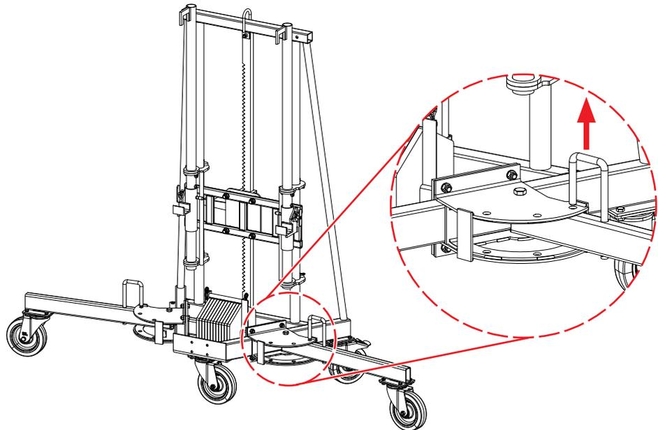
**Step 2** Move the cantilever to the desired position.
