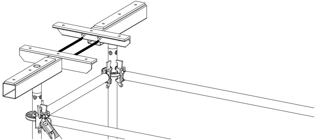
**Step 3** Install the Turning Heads on the opposite side of the MODEX Assembly in the same way.
