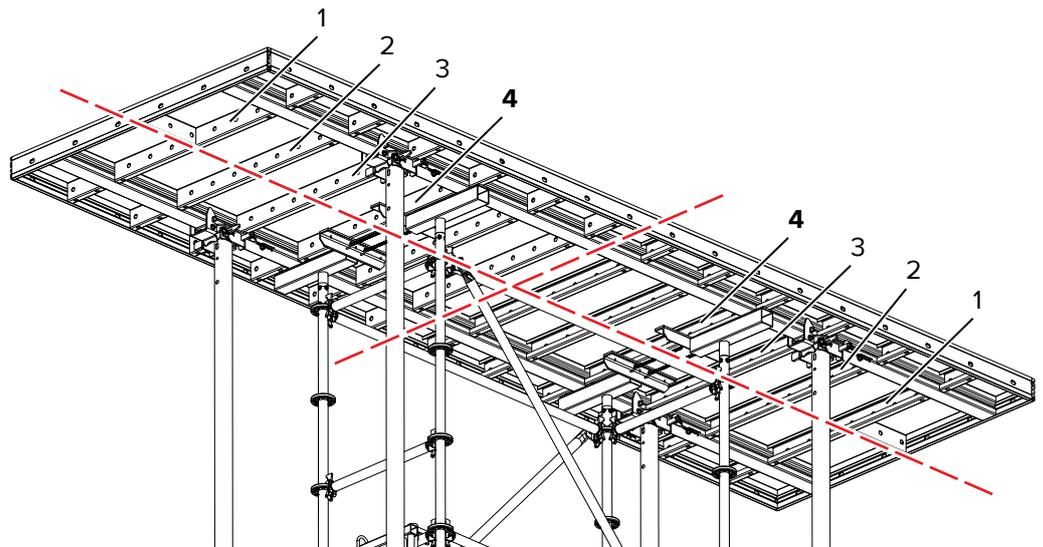
**Step 4** Extend the cantilevers. Do this by pulling out the locking stirrups, extending the cantilevers, and then inserting the bolts again.
