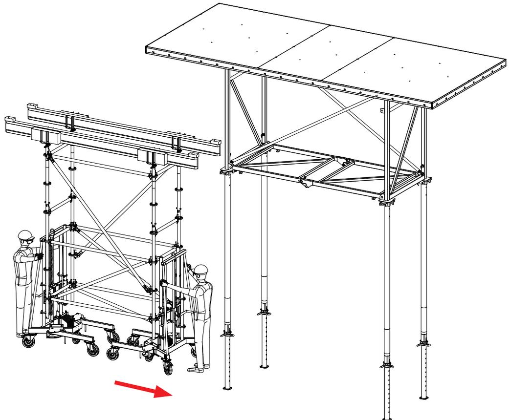
**Step 2** Centre the Positioning Unit under the Extension Frame.
