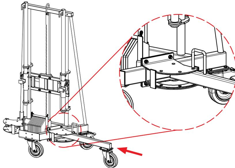
**Step 3** Secure the cantilever with a screw M20x130 and a Nylok nut. Use a spanner SW 30 to do this.
