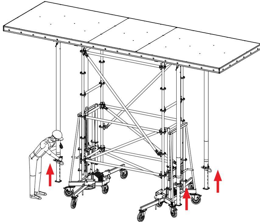
**Step 6** Crank both lifting jacks to evenly lower the Table Form such that collisions with downstand beams or similar parts are avoided. Before setting down, verify that all props are extended the same and that the prop Quick Release Bolts are attached properly!
