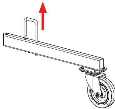
**Step 2** Insert the cantilever into the seat on the Lifting Jack Carriage.
