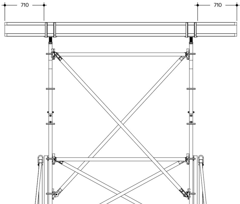
**Step 4** Secure the H 20 K-Beam with boards or wedges to prevent it from tipping to the side.
