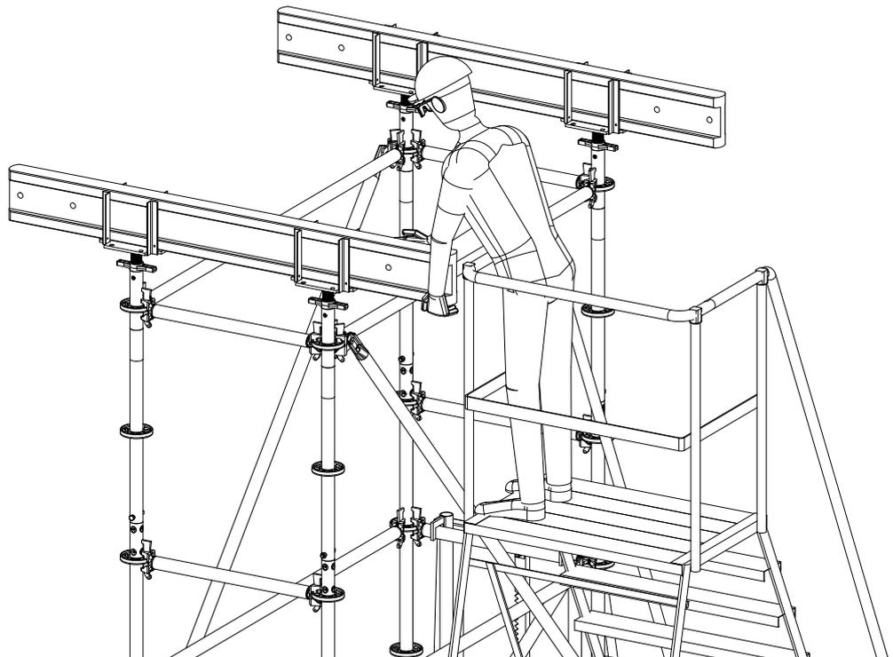
**Step 3** Centre the H 20 K-Beam 190 along the width of the MODEX Assembly.
