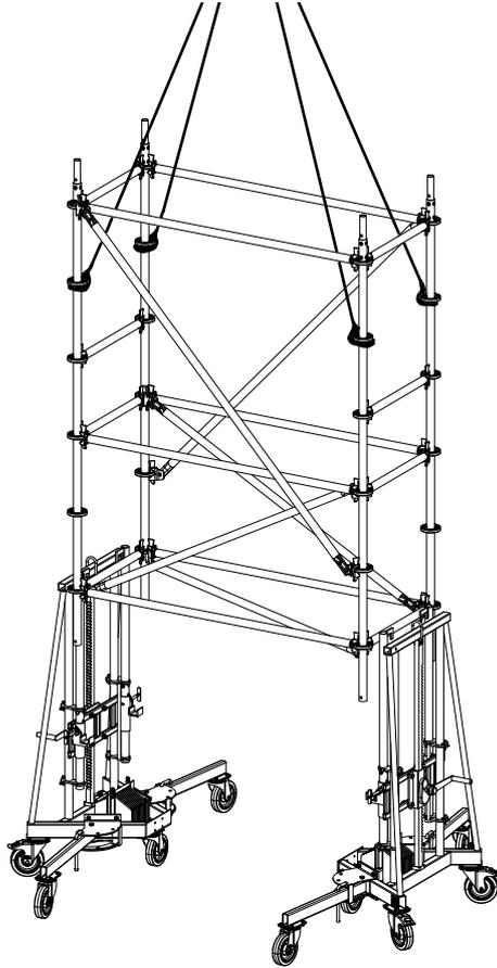
**Step 5** Position the MODEX Assembly and the Lifting Jack Carriages such that the tube ledgers on the MODEX Assembly (**A**) rest in the **middle** of the brackets (**B**) on the Lifting Jack Carriages. Do not detach the MODEX Assembly from the crane yet!
