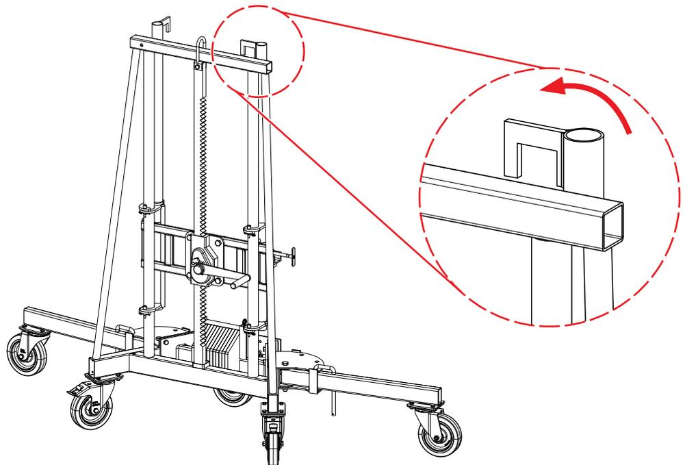
**Step 3** Unlock and turn the second vertical track in the same way.
