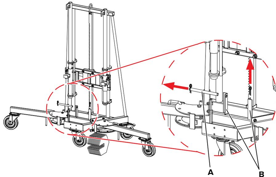
**Step 3** Place all 12no. weights in the bracket, with the slots on the underside.
