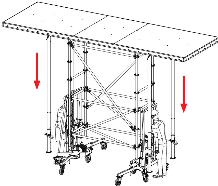
**Step 7** Extend the props such that they are no more than 50 mm off the ground and secure them.
