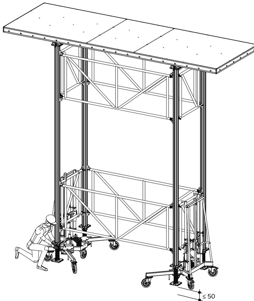
**Step 7** Move the Table Form. Do not exceed the maximum speed of 2.90 km/h (0.8 m/s) for longitudinal transport! Grasp only the steering rods to move the Lifting Jack Carriages!
