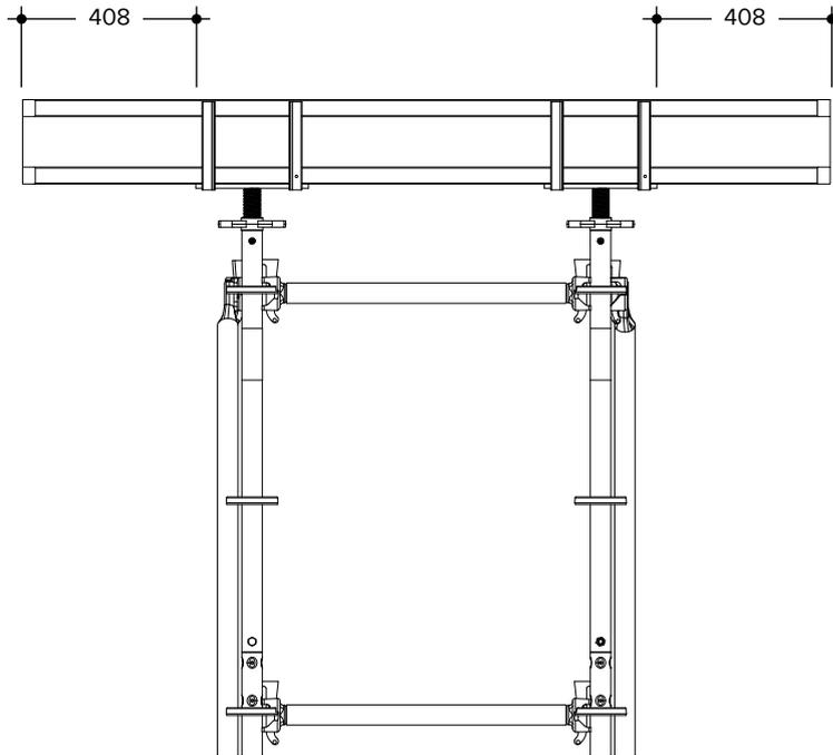
**Step 4** Nail the H 20 K-Beam to the Crosshead Jacks.
