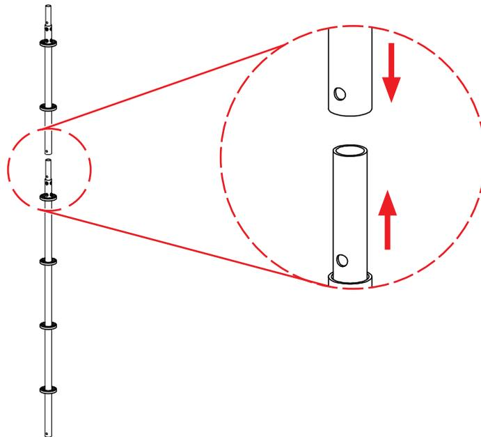
**Step 2** Secure the vertical posts with a screw M12x75 (A) and a nut. Tighten the nut against the shaft of the screw.
