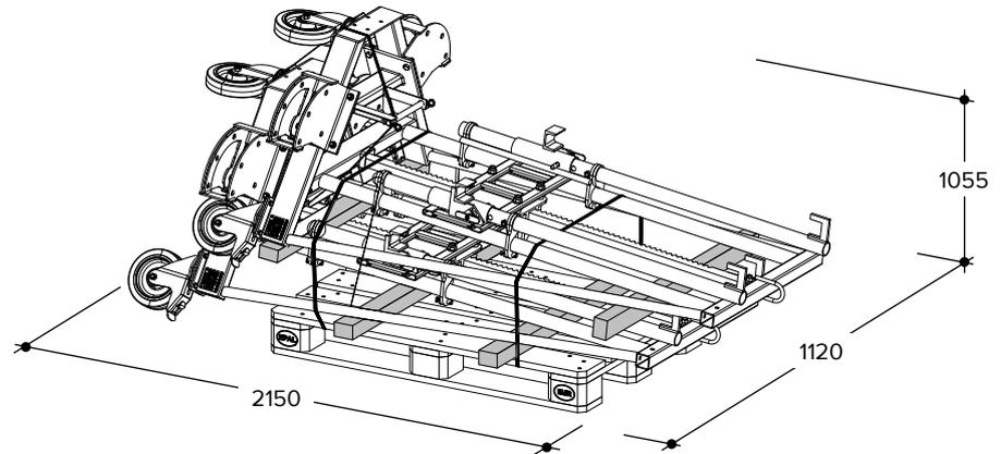
Use a crane to carefully lift the Lifting Jack Carriages off of the pallet. There is a lifting eye (**A**) on the top cross profile of each Lifting Jack Carriage.
