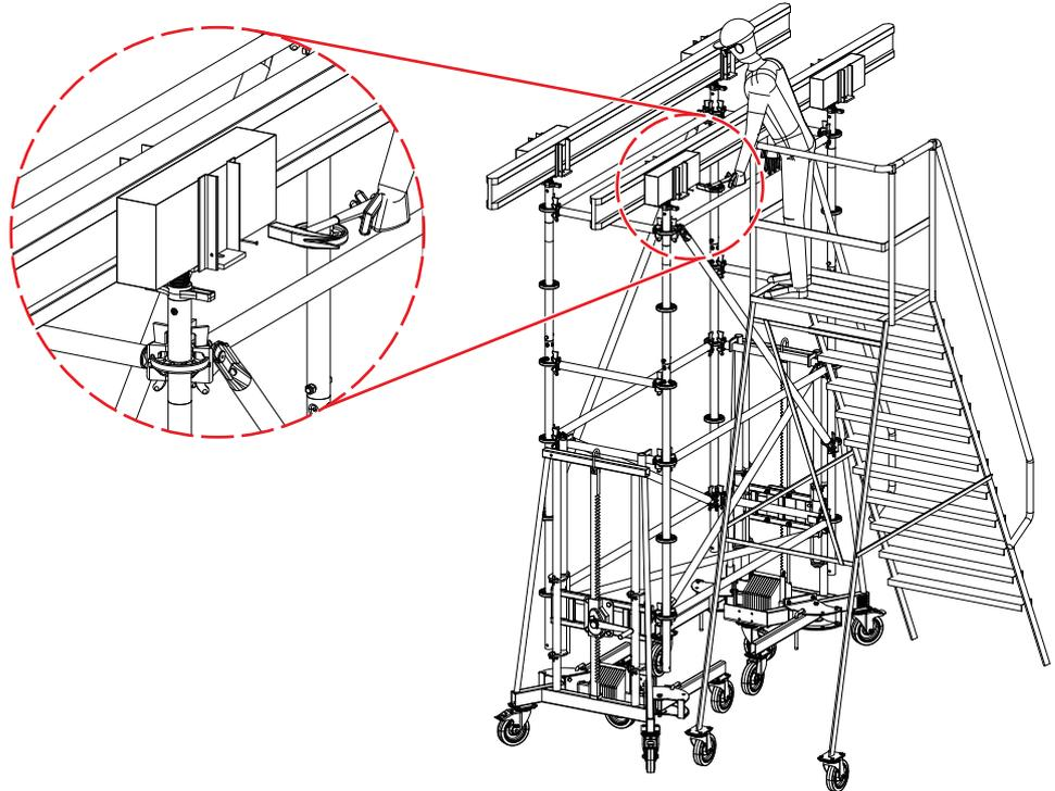
**Step 6** Nail the H 20 K-Beam to the Crosshead Jacks.
