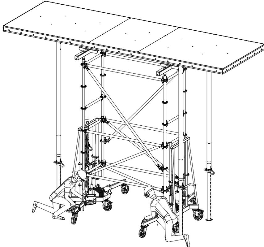
**Step 5** Turn the lifting jacks on both Lifting Jack Carriages clockwise at the same time to lift the Table Form. The props may be no more than 50 mm off the ground when moving! Ensure that all props are extended the same distance.
