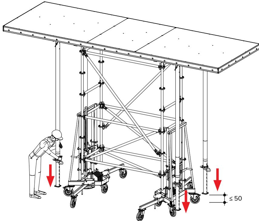
**Step 8** Move the Table Form. Do not exceed the maximum speed of 2.90 km/h (0.8 m/s) for longitudinal transport! Grasp only the steering rods to move the Lifting Jack Carriages!
