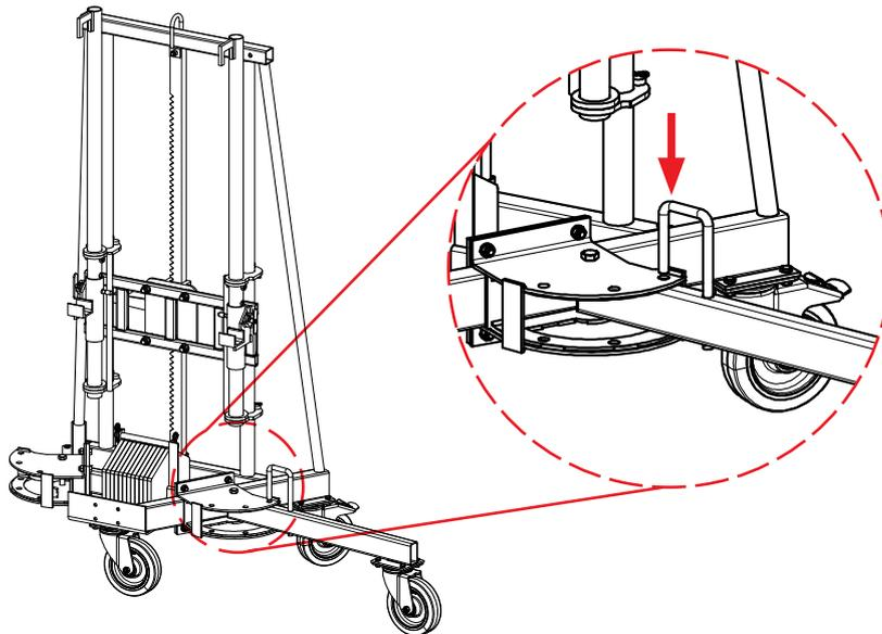
**Step 5** Attach the other cantilever to the Lifting Jack Carriage in the same way.
