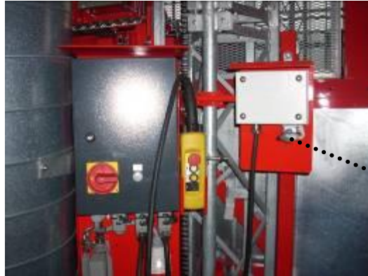
Cable routing at the pivoting gate (platform)
