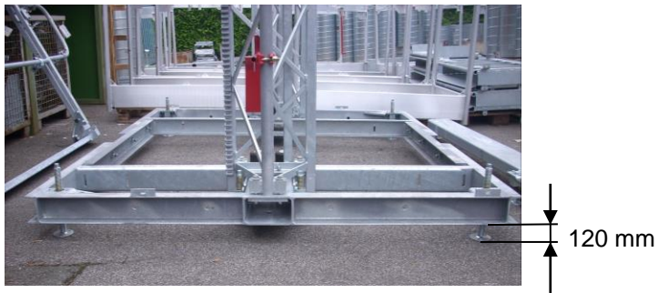
Fig. 12: Spindles of a mast side
