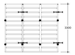
The uppermost tie position on MANTO Panels 330 is needed only when panels are stacked.
