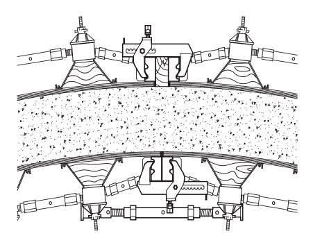
The element connector is easy to use and allows timber adjustments of up to 15 cm
