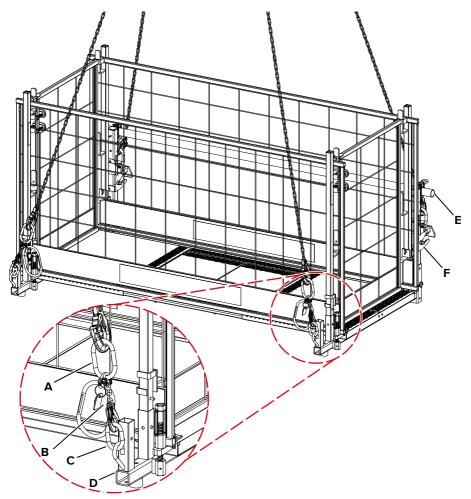
To move a single formwork platform with formwork by crane, attach the other 2no. strands of the chain sling to the larger suspension link (**G**, red) on the Crane Suspension. Never use the Crane Suspension to raise or lower formwork elements!
