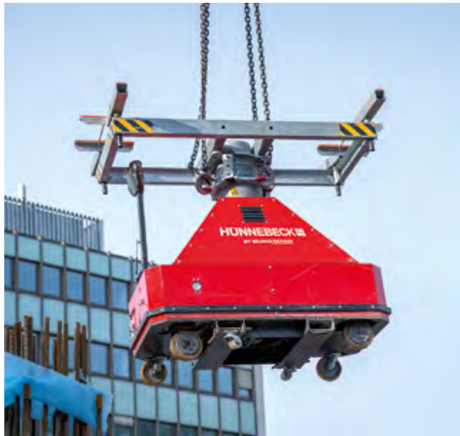
► Safe moving thanks to integrated crane attachment points
