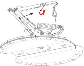
**Step 3** Press the lever on the inside of the base mast into it. This closes the release valve.
