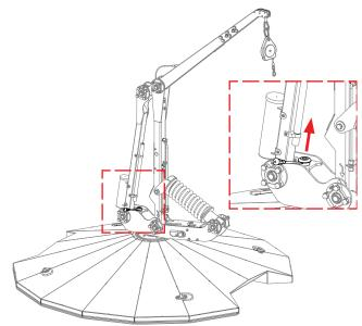
Step 7Connect Body Restraint Device (code:612403) of the PPE to the Fall Arrester 8.00 m.The Falpro – Mobile Fall Protection Anchor is now ready for use
