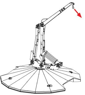
**Step 2** The extension arm of the device retracts towards the base. The rotation lock secures the position of the extension arm automatically.
