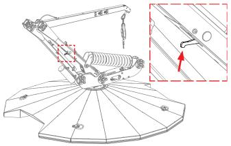
**Step 4** Remove the pump tube from the inside of the push rod. Insert the pump tube into the opening of the pump lever as far as possible.
